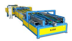
It's mainly for uncoiling, leveling, beading, punching, locking, bilaterally angle steel or TDF flange forming. Because of its small space requirement and easy to install and operate, people also call it "small line 5".
